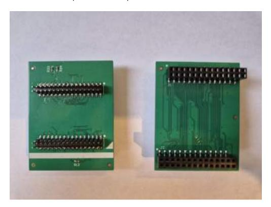
Once you have plugged the memory module onto the adapter and then placed it onto the PROMAN, it should look like this (please refer to the two white markings on the adapter board that indicate correct orientation):
