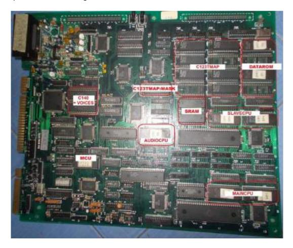
REMOVE all the chips in the following sections: MAINCPU, SLAVE CPU, AUDIOCPU, C140=VOICES, C123TMAP:MASK, C123TMAP and DATAROM.
