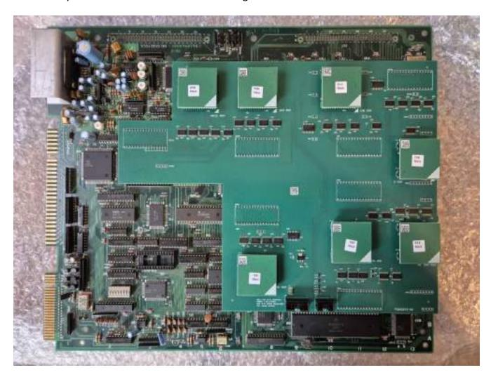
After installing the two multi PCBs to your donor, re-assemble your System 2 stack, and connect the cable between the Video and Main Multi PCBs and also the selector cable to the Main PCB.
