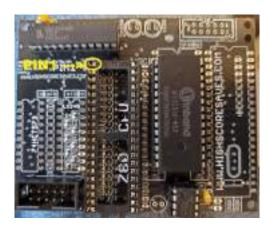
Ensure that nothing is hitting the underside of the new daughter card from your original PCB. Sometimes test points on your PCB need to be bent away.
