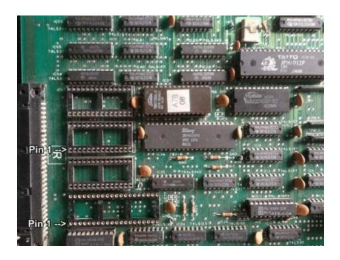
Insert the EEPROM shipped with the savekit and marked as "IC52" at Position IC52. Make sure Pin 1 of the EEPROM is oriented to correctly match Pin 1 on the board. (see pic above)
