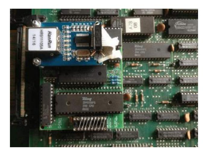
Insert daughter board into the cpu socket of the board where the CPU chip was removed from.
