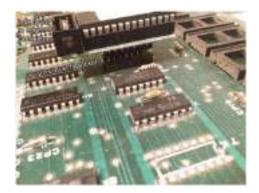
Insert the PROM board labeled with 4A into the socket located at 4A (the 10pin jack must point towards the edge connector of the game board).
