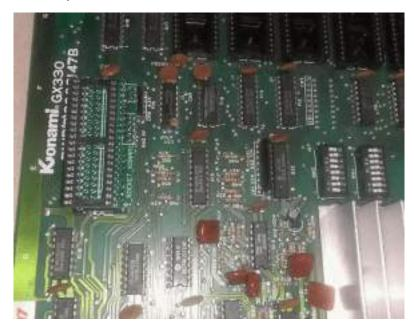
Install the main daughter card like this on top of the adapter. I installed the 6809E before I installed the daughter card. **Again, ensure it is a 6809E or kit will not work**.
