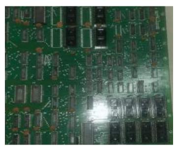
Now, desolder the jumpers at JP1 (D11) and JP2 (F18) and move the pin to 128 from 64 on each one (D11 and F18). If yours are already at 128, great! The pics below show both already desoldered before I move the jumper wire to 128...
