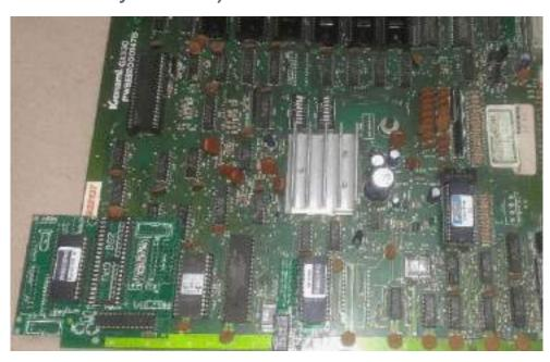
Now we need to install the 6809E adapter UNDERNEATH the main pcb daughter card at E/F 18. This is a 42 pin Konami custom chip. You will have needed to order from Highscoresaves a 6809E to fit on the main daughter card (or have your own. Only a 6809E will work)
