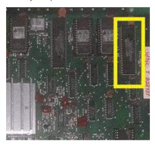
You will need to desolder the prom at C3 and install a new 16 pin narrow socket here –
