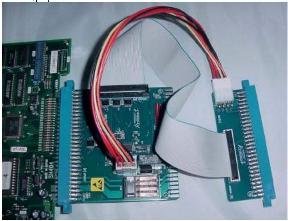
The Master board or board A is the first board selected on power up, then satellite board B
