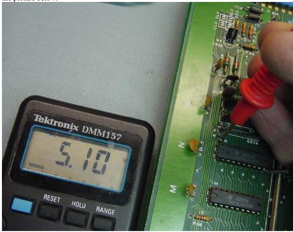
THE VOLTAGE READING SHOULD BE NO LOWER THAT 4.75VDC. If it is lower and you power supply does not have a way of adjusting the voltage to at least that minimum level then we strongly suggest you purchase a new switching power supply like the Happ power supply.
