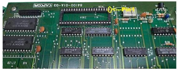
2. Install the z80 onto the daughter card then attach on PCB like this. [Ensure PIN 1 of the z80 is installed with the proper orientation]-
