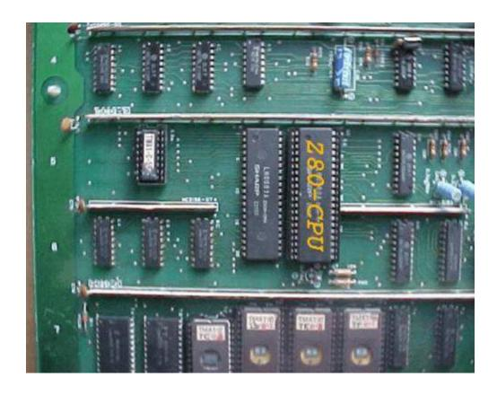
Insert the just removed Z80 chip into the empty 40 pin socket on the High Score Save Kit. Make sure pin-1 is correctly oriented. Pin-1 is marked on the Z80 chip usually by some type of indentation or circle molded into the plastic. The end of the chip with the marking, needs to match up with the
