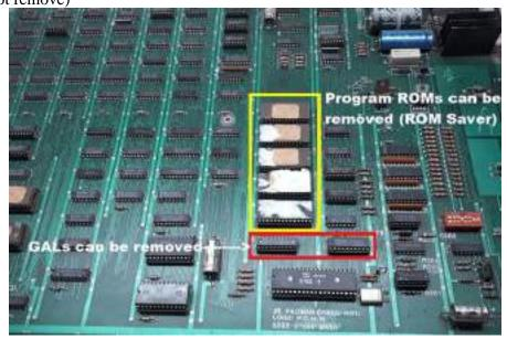
**2.** Remove cpu, plug cpu on savekit, plug kit where z80 was. Note the notch on the z80. Online kit shown as reference. The offline will install the same way.
