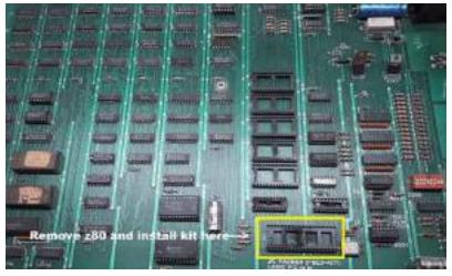
The kit overhangs the pcb a tad on the far side.
