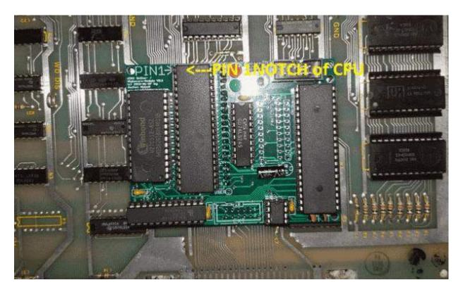
Install save kit on your PCB with the 6502 in same orientation before you placed on the save kit [Ensure PIN 1 of the 6502 is installed in the proper orientation]
