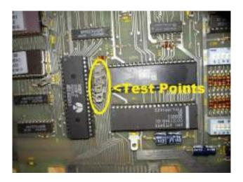
Insert the riser pcb at C2 (where the 6502 was removed from). Note the Pin1 and install like pic below (the riser may be a 40-pin machine socket instead of the small pcb pictured, they work the same to raise the height properly)
