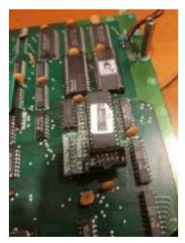
Locate and remove PROM labeled GYC from F6. This us where you installed the socket where the 378C riser board was present (position G7. If not, the LS378 present on the board at this location does NOT need to be removed –
