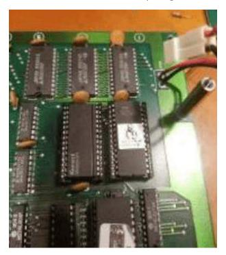
Reseat the Konami custom into open slot on PCB with roms labeled G1/G2. Now place daughter card in g/h 1/2/3. Remember Pin 1 is on the line side of the Konam1 custom chip. See pic below –
