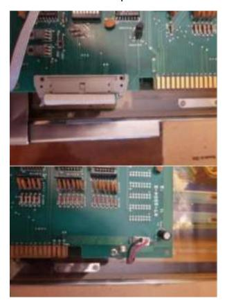
Reinstall PCB in Gyruss game and test. Pay attention to the orientation of the harness to the PCB edge connector. After insertion, check the seating of ALL the daughter board again to ensure proper seating in the socket.
