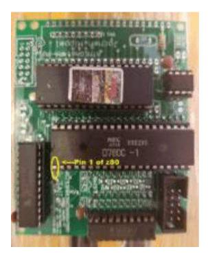
NOTE - Insert CPU into CPU position on CPU PCB, see where PIN1 is by the notch on the z80 itself. CPU board may not fit without bumping into other items on PCB, additional socket may be used as riser in this case. Again, a zip tie may be necessary.
