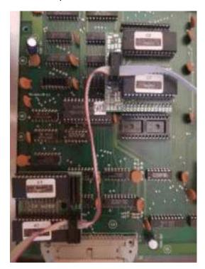
Reassemble PCB stack using included new risers. If you previously had a high score kit installed, the risers used when installing that kit will suffice.
