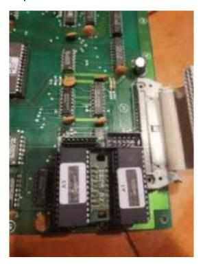
Locate and remove GYB labeled PROM at E3 and LS378 from the socket at F2. In some cases, a LS378 & riser board will be present here instead, in that case, you already removed this and put a new socket in —
