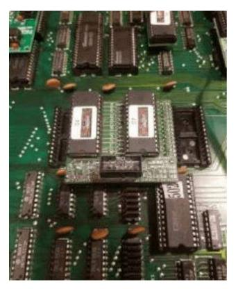
Locate and remove CPU at position F/G 13. Insert in main daughter card of kit as seen below. —
