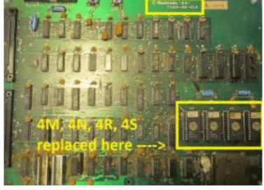
Picture of a 2 PCB stack and where to install –
