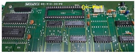
2. Install the z80 onto the daughter card then attach on PCB like this. [Ensure PIN 1 of the z80 is installed with the proper orientation]-
