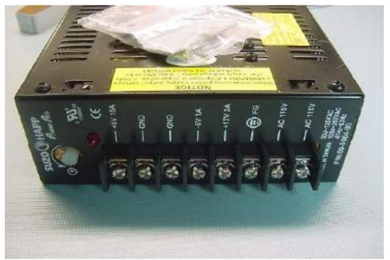
This type of supply has an adjustable +5v (white screwdriver adjustment on left). It can be wired into the 6 pin connector on the selector board as pictured below.
