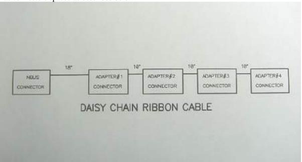
Attach "keyed" ribbon cable connector into NBUS header on selector board as shown.
