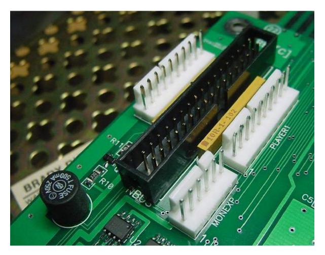
For controls expansion there are two 10 pin headers labeled Player1 & Player2 if extra buttons or joysticks are needed or if you cabinet does not have a control panel harness.
