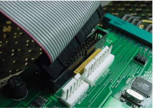
Attach one of the 4 remaining connectors into the NBUS header on the adapter board and One of the 4 power cables into the white header marked power, repeat until all adapters are connected.
