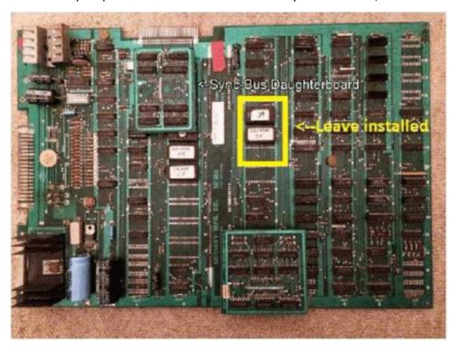
1. Remove your sync bus card and set to the side to install back later. Note its orientation.
