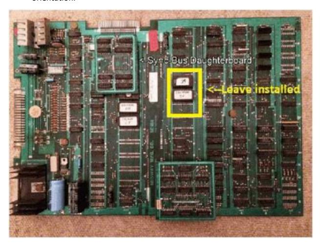
2. Remove z80, plug z80 on save kit, plug 40 pin flat cable where z80 was, plug back sync bus-controller, secure sync bus controller w/ cable tie powerup. If you are installing on a Ms Pac pcb, you will simply replace your existing ribbon cable and daughter card with ours.
