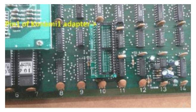
Install a 6809E on the kit and install daughter card on top of the Konami1 adapter. [Ensure PIN 1 of the 6809E is installed the proper orientation]
