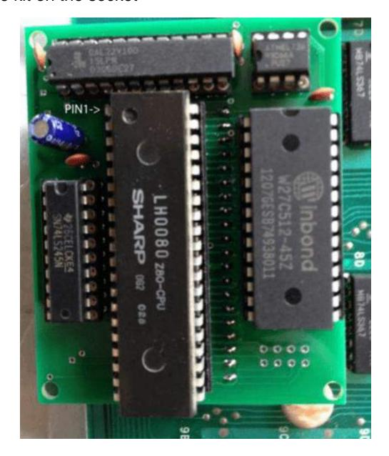
Ensure that nothing is hitting the underside of the new daughter card from your original PCB. Sometimes test points on your PCB need to be bent away.
