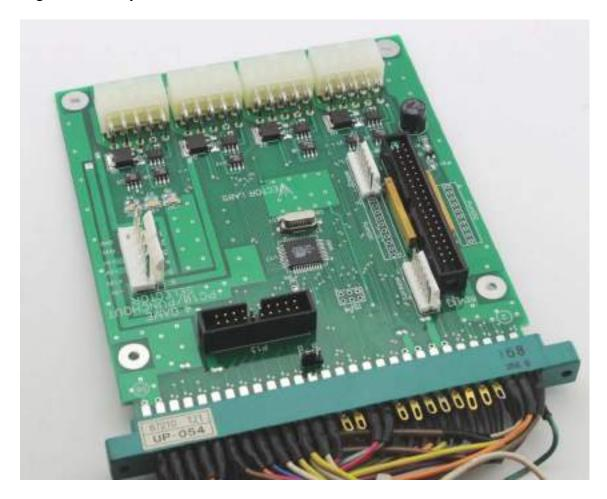
Attach ribbon cable connector that has a strain relief into the NBUS40 header and the black harness connector to P13 on the selector board as shown in the picture below.
