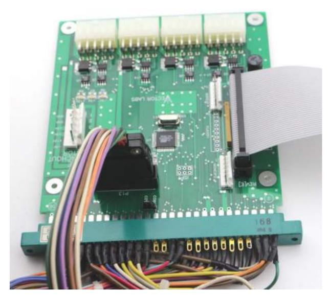
Attach one of the 20 pin ribbon cables from the Playchoice Dual Monitor Adapter to the 20 pin connector on the PC10 game board. Now attach NBUS40 ribbon cable onto the 40 pin header on the adapter board and one of the two power cables into the white header marked power as shown below.
