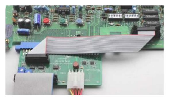
The PC10 dual adapter has separate volume control pots So that you can match volume levels with other adapters.
