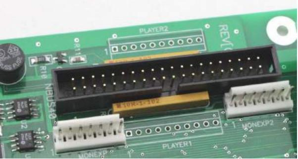
Normally these headers are not installed from the factory, but can be requested free of charge by contacting <a href="mailto:support@vector-labs.com">support@vector-labs.com</a>. The pinout of the connectors is defined below.
