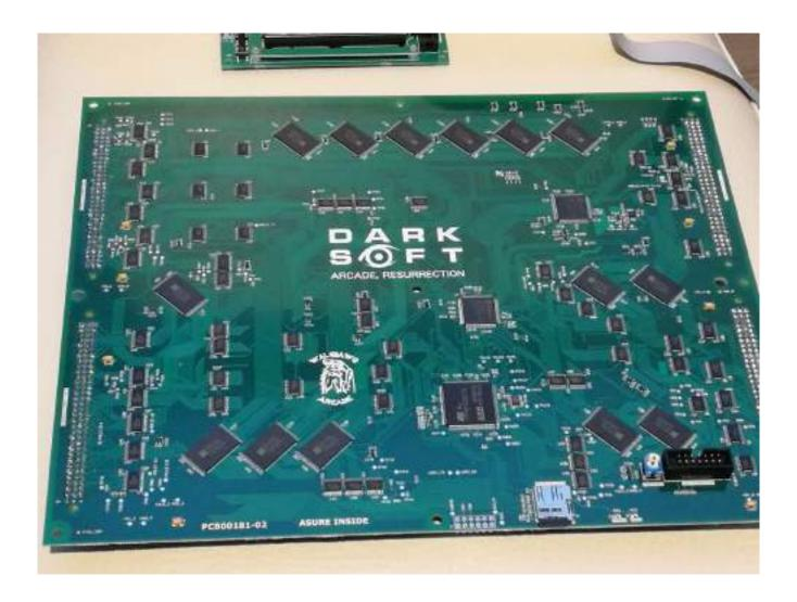
**IMPORTANT!** When installing the Multi you should do it gently, making sure first that everything is properly aligned and then start pushing gently until all the Connectors fit properly
