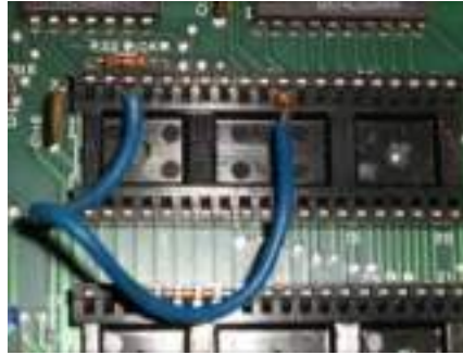
Pins 30 and 38 need jumpered
