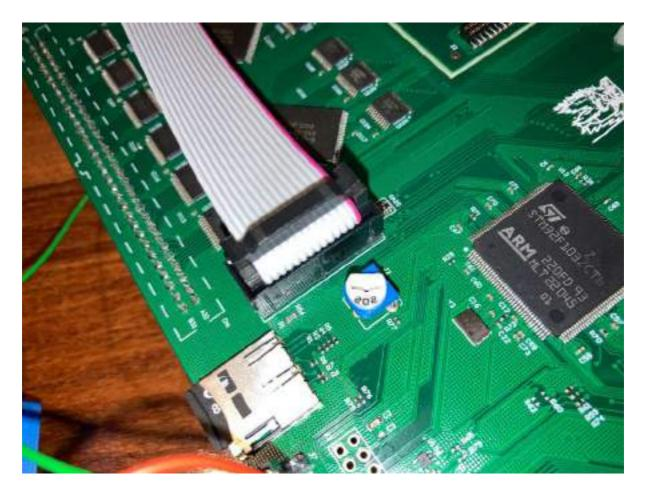
If the contrast is too high or low, there is an adjustment pot on the main Multi PCB (labelled 202, as seen in the photo above) for fine tuning. It's normal for the brightness on the LCD to fluctuate when your voltages are different between machines/superguns.
