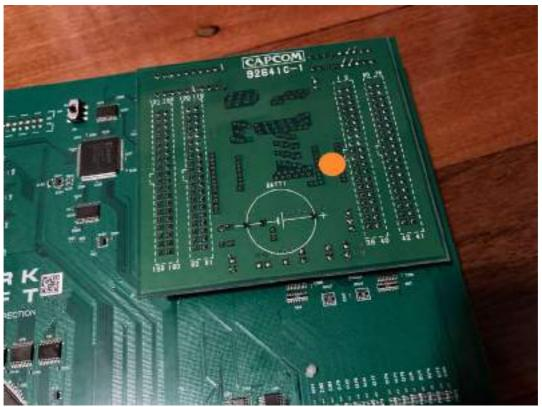
3. **SET C-BOARD SWITCH:** If you are using a C-Board that has just one PAL chip (92641C-1 or 90630C-4) or if it doesn't have the JST connectors for controls, then you need to activate the switch at the top of the Multi PCB to the **"ON"** position.
