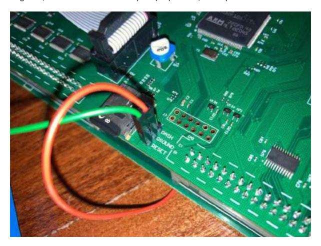
**NOTE:** There is an unused pin in this step labelled "DASH". This pin indicates if the game is 10Mhz or 12Mhz mode. This can be used with future crystal/clock speed add-ons for the multi to denote the native speed of the game.
