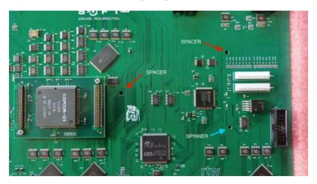
5. **RESET / QSOUND WIRE INSTALL:** The two DuPont wire cables included in the kit are precut, stripped and ready for installation. Before installing to the points of your CPS-1 motherboard, it's recommend you pre-tin both wires and add a tiny amount of solder to the points of your motherboard for an easy flow.
