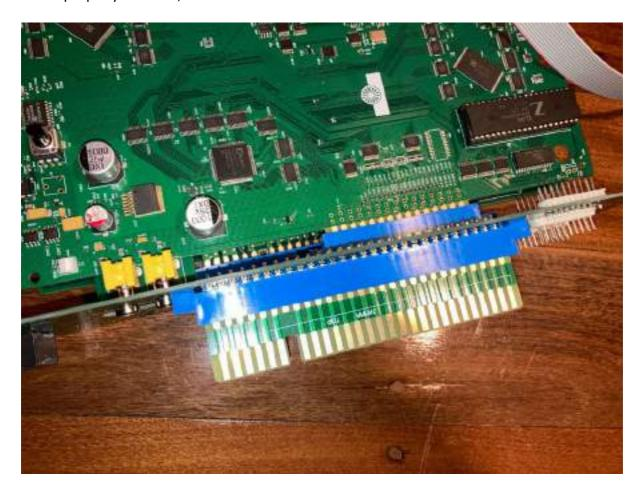
9. **LCD / RIBBON CABLE INSTALL:** Connect the LCD Ribbon Cable to the Multi board in the orientation shown below. Connect the other end to the LCD selector.
