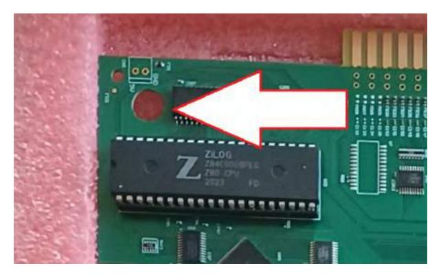
CPS-1.5 games do not use this volume knob, instead there is a potentiometer on the multi PCB to adjust sound output level over JAMMA, but this is ONLY used for games on the CPS-1.5 platform.
