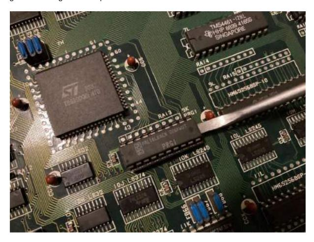
2. **C-BOARD INSTALLATION:** Install your compatible C-Board onto the Multi in the correct orientation. It is important to install the C-Board **BEFORE** installing the multi onto your A-Board as doing it afterwards will flex your multi stack too much and potentially cause damage.
