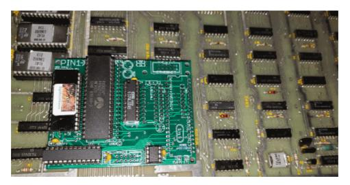
4. Install save kit on your PCB with the 6502 in same orientation before you placed on the save kit [Ensure PIN 1 of the 6502 is installed in the proper orientation]
