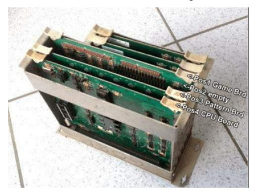
Please always when inserting in the stack it, make sure that the nose of the slots with the notch on the Board (see arrow markings)
