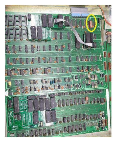
5. Turn all dip switches to OFF on your SOUND PCB. It is the red 8 dip bank circled above.
