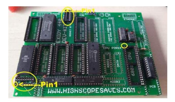
5. Now, install the main daughter card onto your PCB. Ensure the pins line up properly in all 3 sockets and press firmly to ensure good connection.
