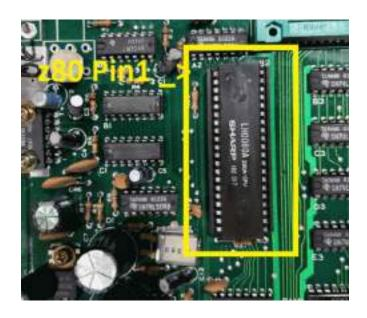
2. Insert riser socket (Needs to clear caps on the left for kit to sit properly) [Ensure PIN 1 of the z80 is installed with the proper orientation]-
