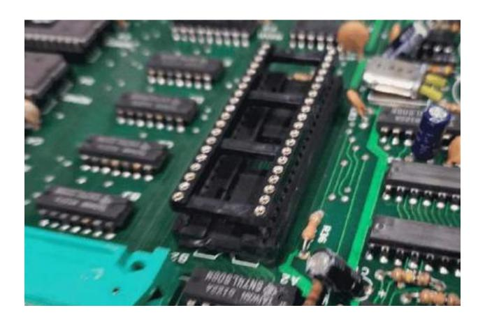
3. Insert daughter board into the cpu socket of the board where the CPU chip was removed from. Place z80 on kit.
