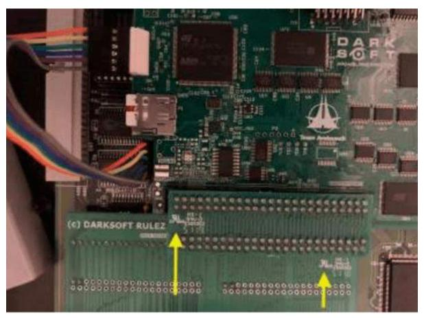
All versions of the 'Champion Edition' multi come with firmware installed that allows you to use original untouched and unpatched ROM sets. For this to happen, you need to plug a "key writing" cable between the main PCB of the kit and the JST NH connector marked CN9 on your 'B' Board. If you have one of the older type 'B' boards, then you'll need to solder 4 wires between this connector on the main PCB of the kit and CN2 of your 'B' Board (see "Additional Soldering Instructions" section below).
