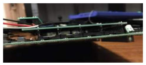
2. **BEFORE** installation of the main PCB, insert the two plastic spacers. Some spacers will require screws, otherwise the spacers will simply "push in".
