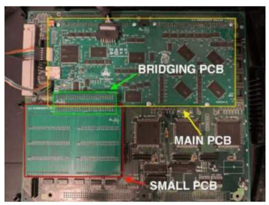
**IMPORTANT!** When installing these PCBs, you should make sure first that everything is properly aligned and then start pushing very gently until all the pins are inserted into the ROM or motherboard sockets. Please be careful and take your time.
