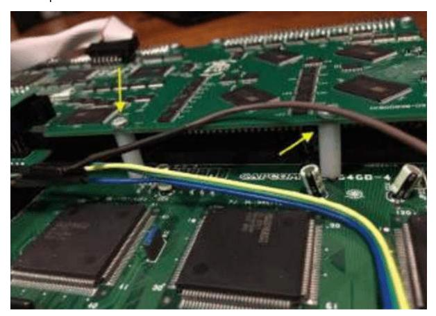
3. After inserting the spacers, install the main (larger) PCB. There are no longer any long pins and the board will easily slot into place on the sockets of the 'B' Board.
