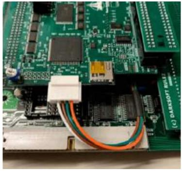
Also, for reference, in the photo below, CN2 A32 is white, A31 is green, A30 is brown, A29 is orange. If your 'B' board has a resistor between A32GC32, leave it installed.
