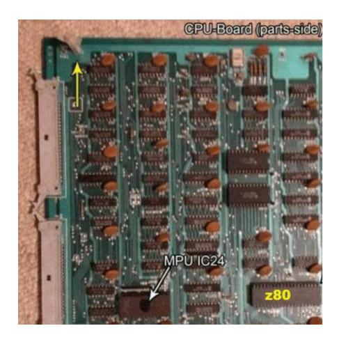
Insert the Z80 CPU that you just removed into the socket of the Multi High Score Save kit
