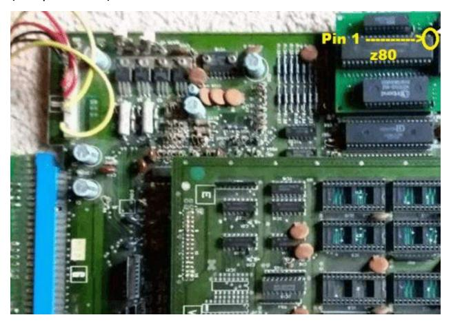
Now insert the Multi Sound Module into the empty socket at location IC52.
