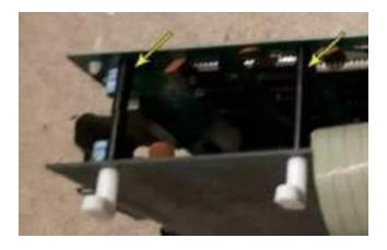
Mount the Game PCB on top of the Video PCB using the original nylon spacer.
