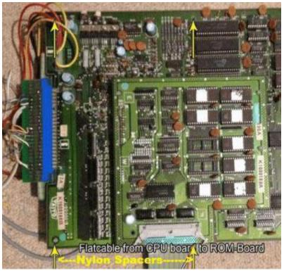
Disconnect the flat cable connectors from the VideoBoard to the CPU Board
