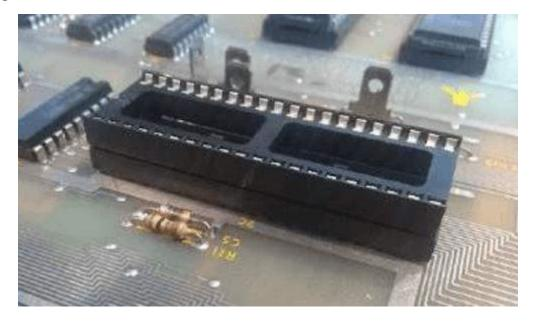
The main daughter card will sit on top of the riser. Pic below shows the needed height to clear test points –
