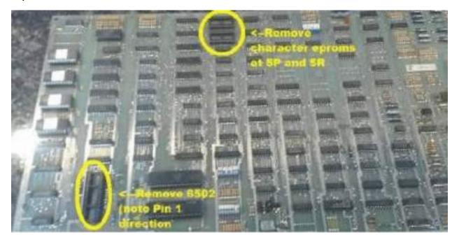
Remove the 6502, plug 6502 on save kit, then, plug kit where 6502 was. Note the notch on the 6502. Online kit shown as reference. The offline will install the same way.
