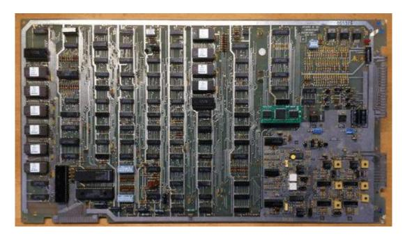
This is the 6502 that you will want to remove, install the riser and the kit, then populate the 40-pin socket on the kit with the 6502 you just removed from your pcb. Described below.
