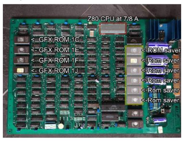
Remove the z80, plug z80 on the main daughter card save kit, then, plug kit where z80 was. Note the notch on the z80.
