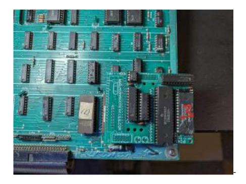
Verify that the kit is seated fully in the socket and nothing is touching the underside -
