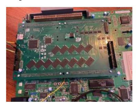
5. The final installation step is to connect the Reset and Audio wires to the Multi. Using the colour coding shown in this guide; Green is **RESET** and Yellow is **AUDIO**. The colours of the wires included in your kit may be a different colour, so please be sure to check.
