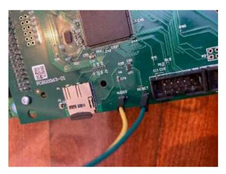
6. Now connect the selector of your choice. The 10gpin connector is for OLED and the 14gpin connector is for a traditional LCD screen. Either selector will work standalone, but there's also no danger in using both at the same time. The screens will refresh in unison in this case.
