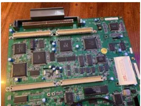
2. Next, we need to install a wire for Auto Reset. Solder one of the included DuPont wires to Pin #8 of IC12. Lightly tin both the DuPont wire and Pin #8 with solder andgently tap it down to make a strong connection. Whilst this step is optional, if this wire is not installed, you will need to power cycle your Multi for the game to load.
