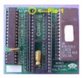
4. Install save kit on your PCB with the 6502 in same orientation before you placed on the save kit [Ensure PIN 1 of the 6502 is installed in the proper orientation]
