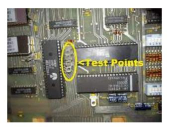
Insert the riser pcb at C2 (where the 6502 was removed from). Note the Pin1 and install like pic below (the riser may be a 40-pin machine socket instead of the small pcb pictured, they work the same to raise the height properly)
