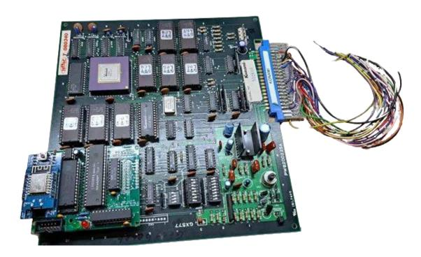
Ensure that nothing is hitting the underside of the new daughter card from your original PCB. Sometimes test points on your PCB need to be bent away.
