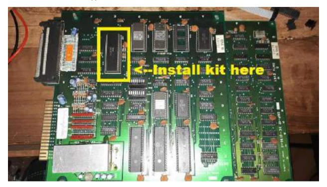
2. Remove the 40 pin 6502 and install on the kit. Note the proper orientation.
