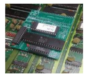
Open stack to reveal CPU pcb (you can remove eproms as shown on row 2, the 5F and H, and the prom at 6E)
