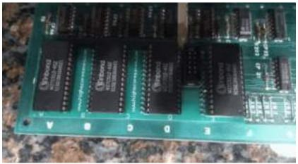
3. Note how the silk-screened letters on the kit aligns with your game pcb. This ensures you install in the proper direction.
