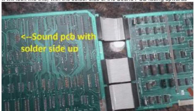
2. Now, you will take the Graphics PCB and fold it UNDER the Super CPU PCB. Those are solder side to solder side. Your original standoffs are still being used.
