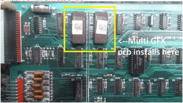
3. Insert firmly and ensure pins are aligned to each socket
