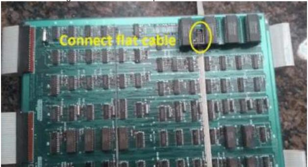
After insertion, check the seating of the daughter boards again to ensure proper seating in the sockets.
