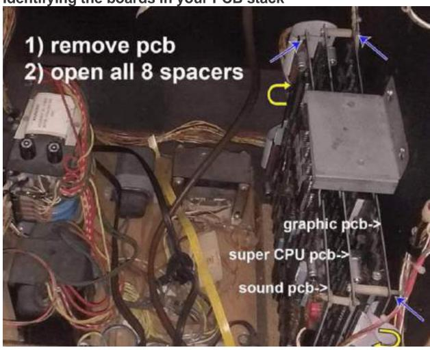
Pic of the boards "spread out" (Ribbon cables stay attached)
