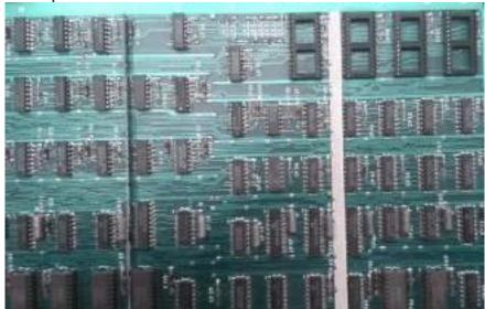
2. Insert the daughter card in the sockets. Be careful and ensure that each pin of the headers are aligned properly with the sockets you are installing in.
