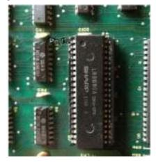
2. Install the z80 onto the daughter card then attach it to PCB like this. [Ensure PIN 1 of the z80 is installed with the proper orientation]-
