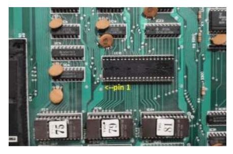
Install the z80 onto the daughter card then attach it to PCB like this.
