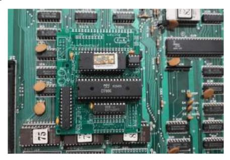
Ensure that nothing is hitting the underside of the new daughter card from your original PCB. Sometimes test points on your PCB need to be bent away.
