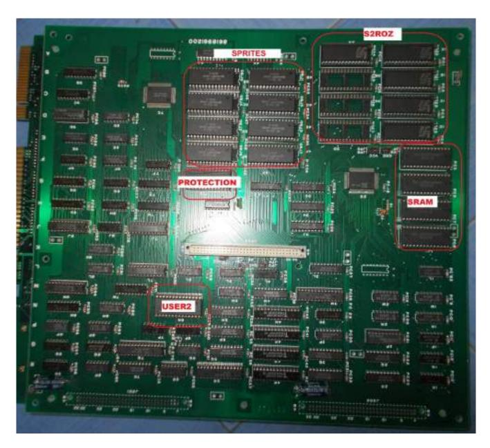
Once you have removed the GND plates that sit below the multi PCB in the MAIN PCB, adjusted the jumpers on both Video and Main PCB and have removed the Mask Roms on both Video and Main PCB, you can proceed to installing the multi.
