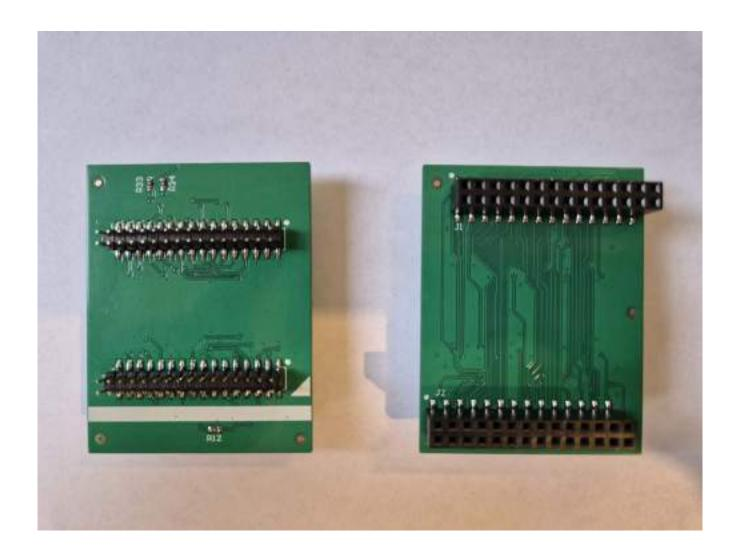
Once you have plugged the memory module onto the adapter and then onto the Proman, it should look like this (please refer to the two white markings on the adapter board that will indicate if it's inserted properly):
