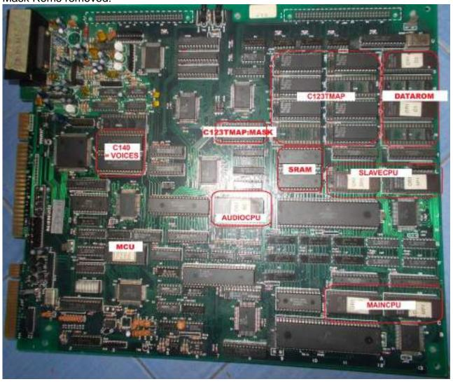
DO NOT REMOVE the chips in SRAM or MCU. You only need to remove the chips in the sections: MAINCPU, SLAVE CPU, AUDIOCPU, C140=VOICES, C123TMAP:MASK, C123TMAP and DATAROM.
