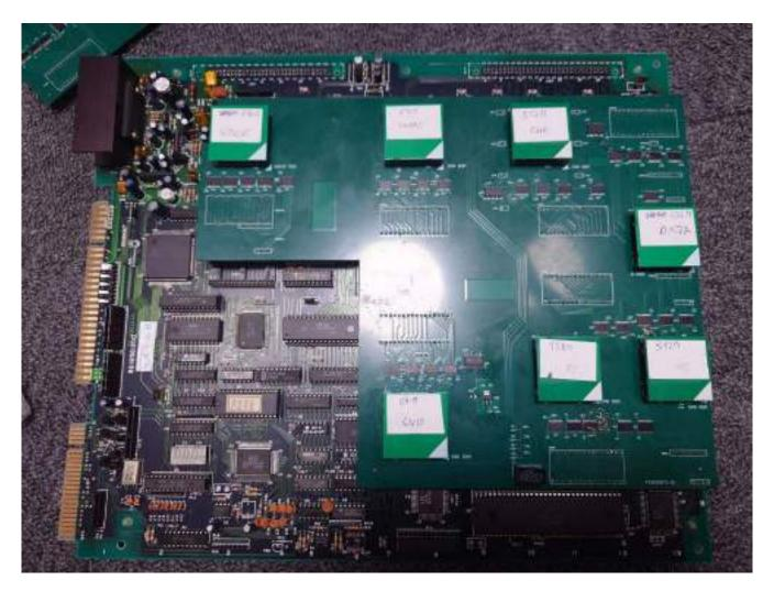
In this case again, as you can see, the PCB for the Main PCB has 7 memory modules, instead of many EPROMS. These memory modules can be unplugged and programmed separately. Note that each memory module has a white triangle on the lower right hand corner. Make sure that you align these with the triangles on the main PCB.
