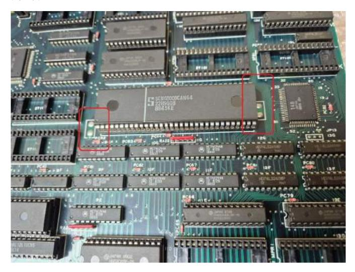
We can now proceed to setting up the Video PCB. In this one, you just need to adjust the jumpers and remove the Mask Roms.
