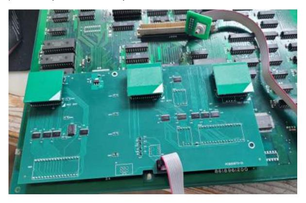
As you can see, the PCB for the Video PCB has only 3 memory modules, instead of many EPROMS. These memory modules can be unplugged and programmed separately. Note that each memory module has a white triangle on the lower right hand corner. Make sure that you align these with the triangles on the main PCB.
