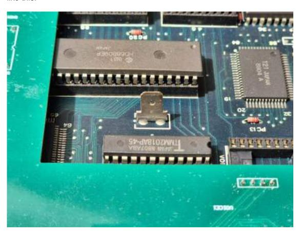
In some cases those GND plates are not mounted in factory, but if they are, you should either remove them or bend them. Notice that this only applies to the MAIN PCB of the (the one with MAINCPU and SLAVECPU), and if any you will find 2 or 3 that are just below the PCB of the multi. In some cases like below, they are not even mounted in the area that could collide with the multi.
