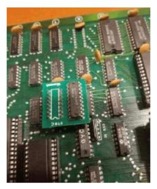
Insert PCB with rom labeled F6 into socket you installed at F6 –
