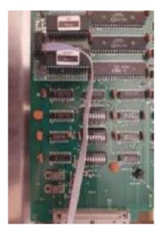
Ensure PCB interconnect ribbon cable and power cables are reattached –
