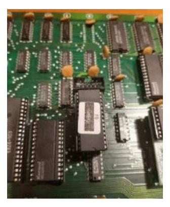
Locate and remove GY6 and Konami custom chip at g/h 1/2/3 -
