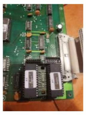
Locate and remove GYB labeled PROM at E3 and LS378 from the socket at F2. In some cases, a LS378 & riser board will be present here instead, in that case, you already removed this and put a new socket in —
