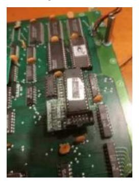
Locate and remove PROM labeled GYC from F6. This us where you installed the socket where the 378C riser board was present (position G7. If not, the LS378 present on the board at this location does NOT need to be removed –
