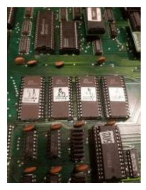
Insert board with roms C7/C8 at sockets located at C7/C8, leaving C6 and C9 sockets empty –  $\,$
