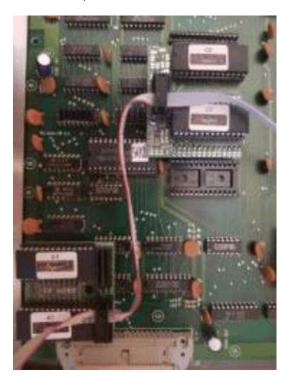
Reassemble PCB stack using included new risers. If you previously had a high score kit installed, the risers used when installing that kit will suffice.
