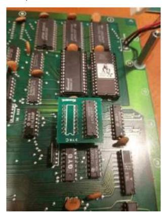
Insert PCB with rom labeled F2 using both sockets at F2/E2 -
