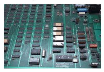
The Conversion Jr Pacman pcb is very similar, however, it does not plug into a standard Pacman (or Ms. Pacman) cabinet like the FIELD pcb above. It uses a DC power pcb...also pictured below.
