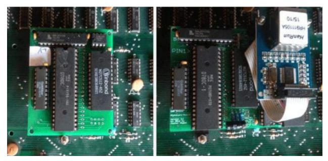
Now carefully plug the save kit on the socket of the former custom CPU jack (the plug of the save kit fits only in the correct direction into the jack)
