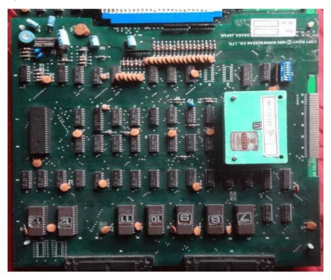
Remove the upper board (CPU board) and remove all screws of the cyan custom CPU block
