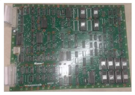
Remove the 12 eproms as shown here and set to the side, they are no longer needed.
