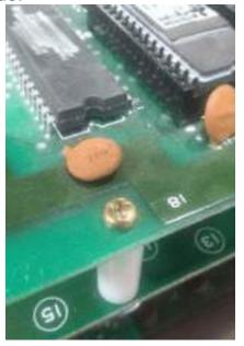
Disconnect the ribbon cables from the top pcb. You should end up with how it looks in the picture below. The Program roms and 2032 cell battery can be removed.
