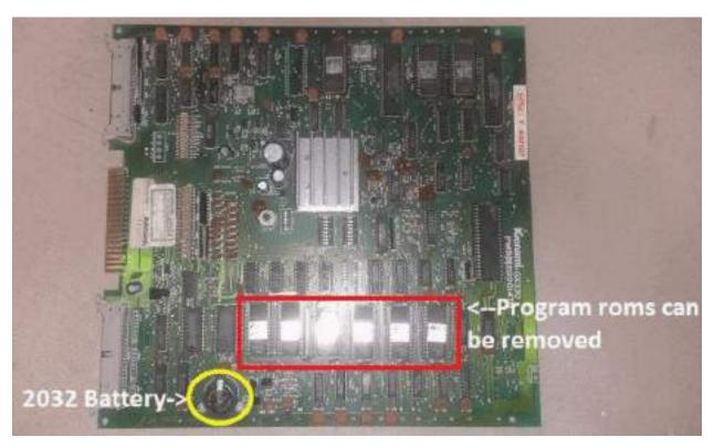
You will need to desolder the z80 and add a 40 pin socket (if not already done) at A/B 18. Ensure you have another z80a to replace or do a damn good job desoldering the one on your pcb...
