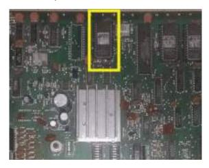
With a new socket installed, you will add the SOUND A/B 18 pcb of the kit. It will look like this
