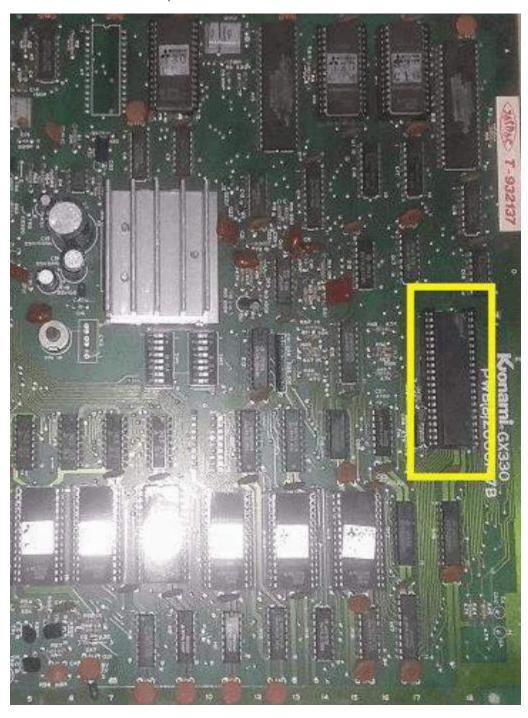
Remove the 42 pin custom. Set it to the side, it is no longer needed. Install the 6809E adapter like this –
