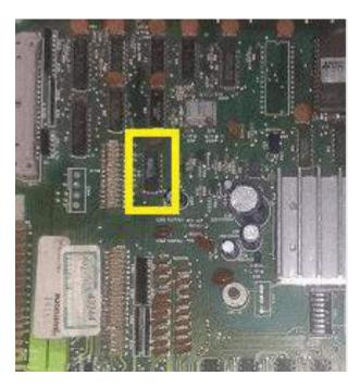
You will need to remove the eprom at A9 and install the new Voice pcb A9 -
