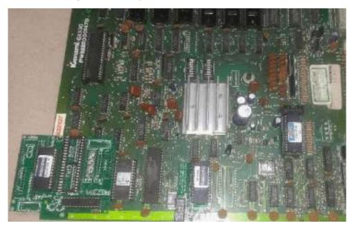
Now we need to install the 6809E adapter UNDERNEATH the main pcb daughter card at E/F 18. This is a 42 pin Konami custom chip. You will have needed to order from Highscoresaves a 6809E to fit on the main daughter card (or have your own. Only a 6809E will work)
