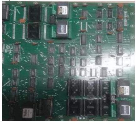
Last but not least....you need to install the ribbon cable to connect all the daughter cards. You can see in the pic that there are 3 connections on the top pcb and there is a long part of the cable that goes around the top of the pcb to the bottom pcb. Feed this near the edge connector as shown. If your provided ribbon cable "isn't long enough", you have it backards.;)
