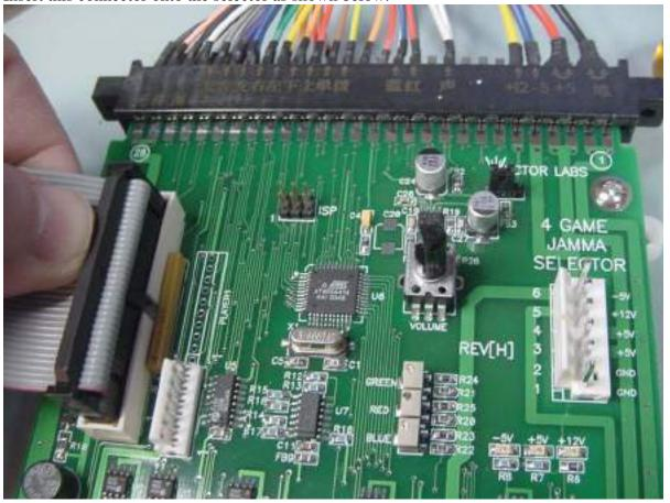
Connect one of the four remaining connectors onto the adapter as shown.
