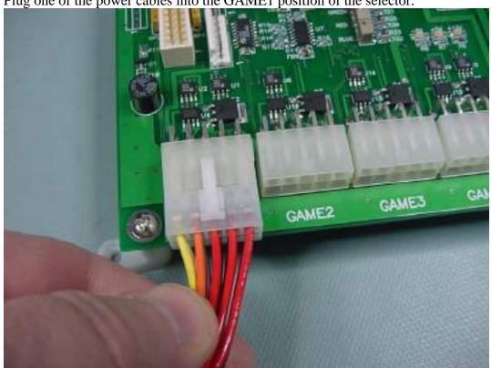
Plug the other end onto the adapter & PCB that you want to be the first on power up.
