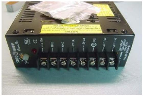
This type of supply has an adjustable +5v (white screwdriver adjustment on left). It can be wired into the 6 pin connector on the selector board with the optional cable pictured below.
