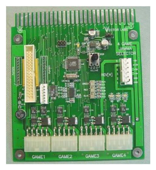
For alternate controls expansion there are places to mount two 10 pin headers labeled Player1 & Player2 if extra buttons or joysticks are needed or if your cabinet does not have a way to connect via the control panel harness.
