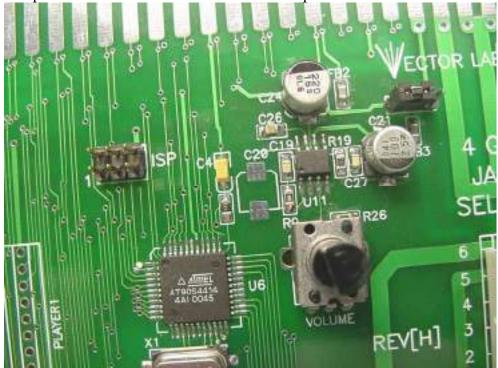
While using a Nintendo adapter with the selector the video will be inverted so that it displays properly on the monitor. There are RED, GREEN and BLUE trimmer pots on the selector that can be adjusted if necessary as pictured below.
