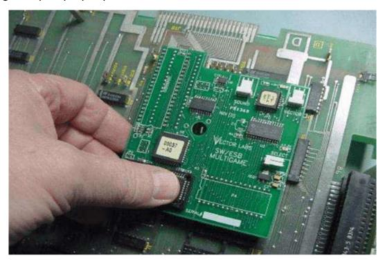
Reinstall 68B09E processor into socket on top of main kit board making sure that the "notch" is towards you as shown below.
