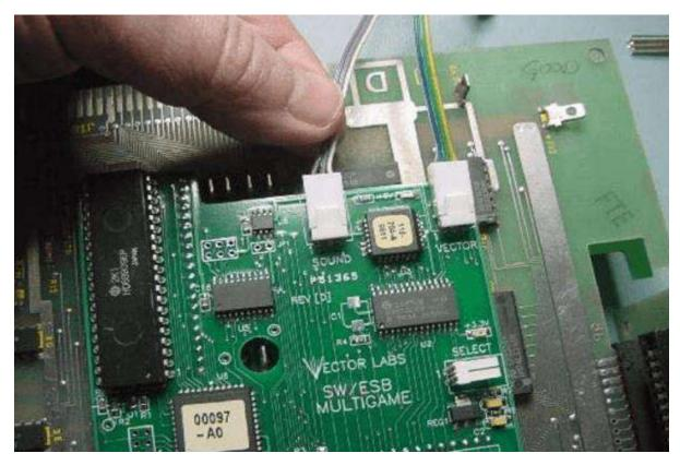
Flip the boardset over and remove the vector Eprom from socket (1L).
