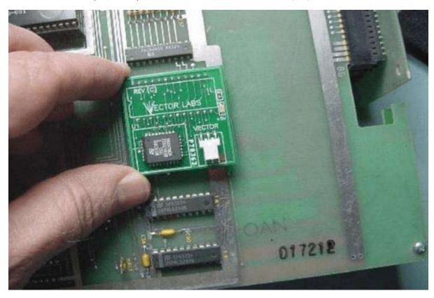
Install the 3 pin cable yellow, green, blue into the white male connector as shown.
