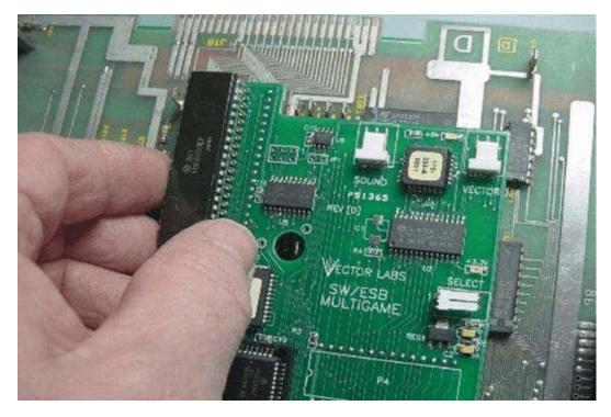
Install both 3 pin cables as shown below, The violet, grey, white into the connector labeled "SOUND" and the yellow, green, blue into the connector labeled "VECTOR"
