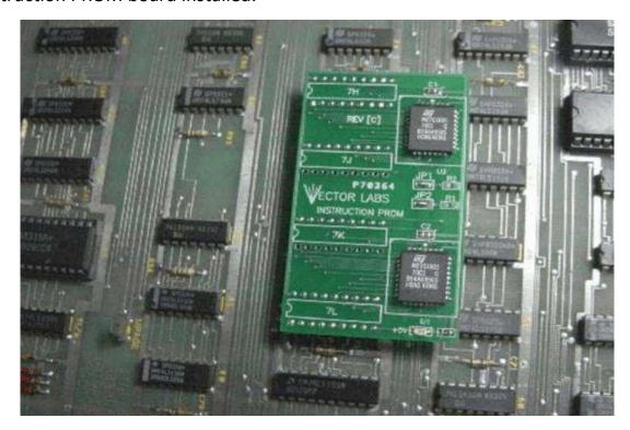
Remove 68B09E processor (2C), NVRAM X2212 (1E) and Eproms from all 5 locations (1F, 1H/J, 1J/K, 1K/L, 1M) as shown below.
