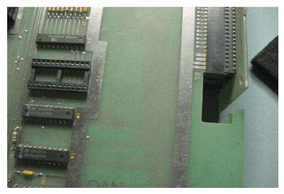
Install the Vector prom replacement board into socket (1L) as shown below.
