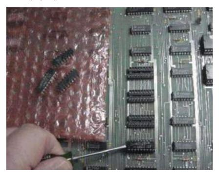
Be careful aligning the pins when installing the Instruction PROM board as shown below.
