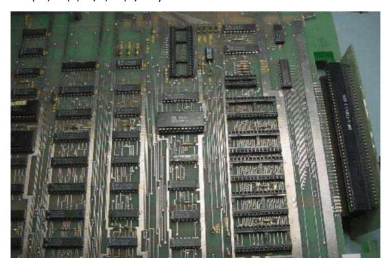
Install kit main board into processor socket 2C & Eprom sockedt 1F being careful to align the pins properly.
