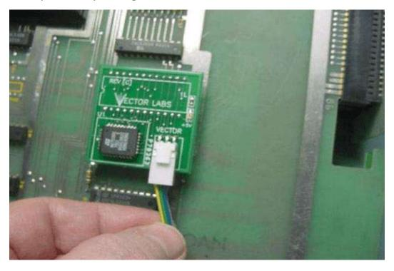
Flip boardset back over and set aside. Remove 68B09E processor from sound board socket location (3K) and Eproms (1J/K & 1H as shown below.
