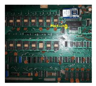
3. Ensure that nothing is hitting the underside of the new daughter card from your original PCB. Sometimes test points on your PCB need to be bent away.
