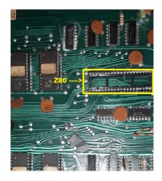
2. Install the z80 onto the daughter card then attach it to PCB like this. [Ensure PIN 1 of the z80 is installed with the proper orientation]-
