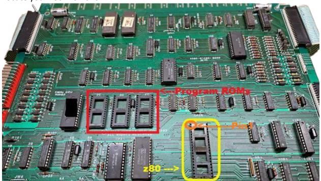
2. Install the z80 onto the daughter card then attach on PCB like this. [Ensure PIN 1 of the z80 is installed with the proper orientation]-
