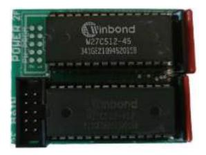
On the CPU board you should have removed the EPROM at 3H. You should have also removed the 2 PROMS at 2F and 2E.
