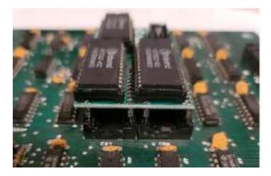
Press DOWN firmly from the top of the board and avoid pressing at an angle to avoid bending any pins.
