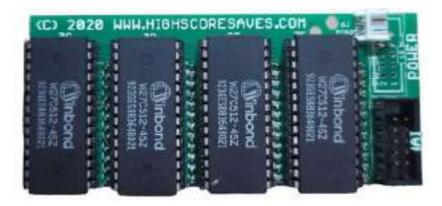
Install this board so the copyright text is furthest away from the edge of the Video PCB.
