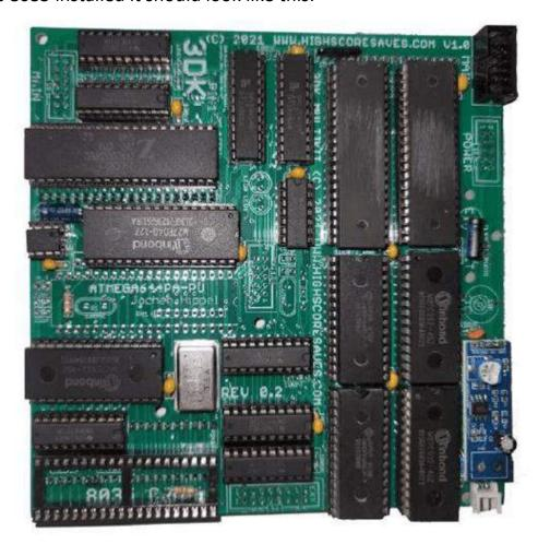
Take your time with this daughter board as it's large and there are a lot of pins! When you press down, you're going to put the pressure on the Z80 and 8035 portion of the daughter board. Make sure you are pushing DOWN and not at an angle.
