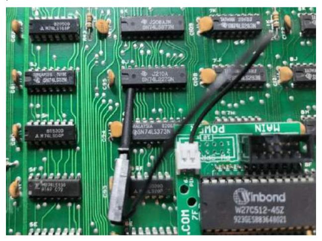
**Optional:** If you plan on keeping the PCB with the kit on it, you can always cut the grabber off and solder it directly to the pin.
