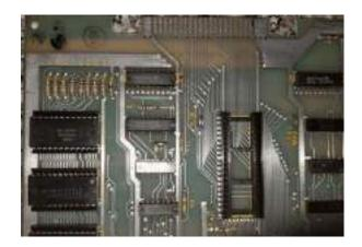
4. Install save kit on your PCB with the 6502 in same orientation before you placed on the save kit [Ensure PIN 1 of the 6502 is installed in the proper orientation]
